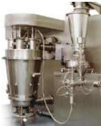
**Figure 1:** Fluid bed dryer for the continuous drying of pharmaceutical granules
