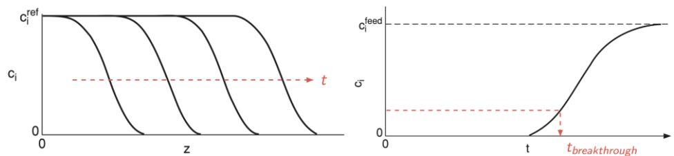
Figure 1 – Concentration profiles (left) and breakthrough curve (right) of an IX column.
