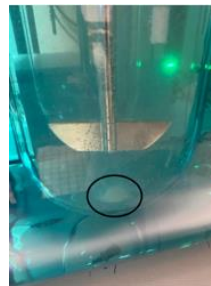
Figure 1 – A vessel used for dissolution testing of tablets
